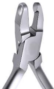
Article# OI8-134 Hole Punch Plier Creates half-moon cutouts in clear aligners to allow space for bonded buttons used for elastics
