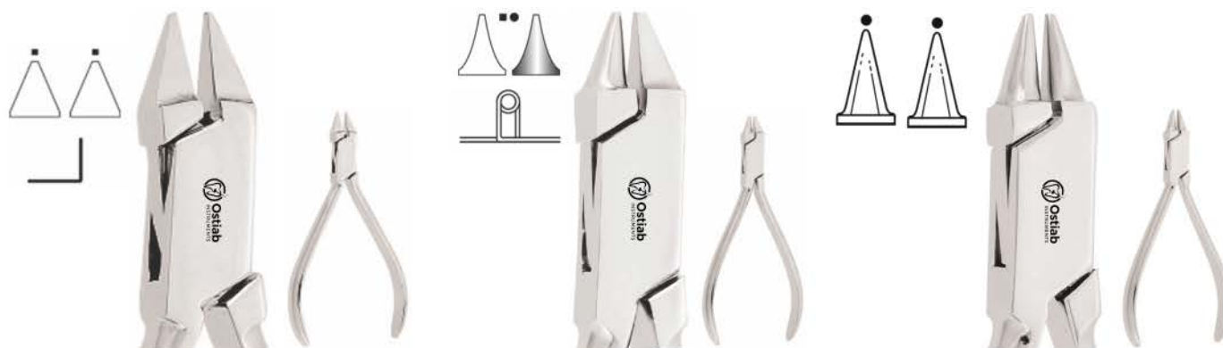
Article# O18-073 Adams Plier Adams pliers for bending wire arches and bends right angles for wires up to .022", .025 tip to beak. Length 13cm
